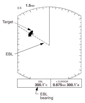
Figure 2-9 Measuring bearing by the EBL
